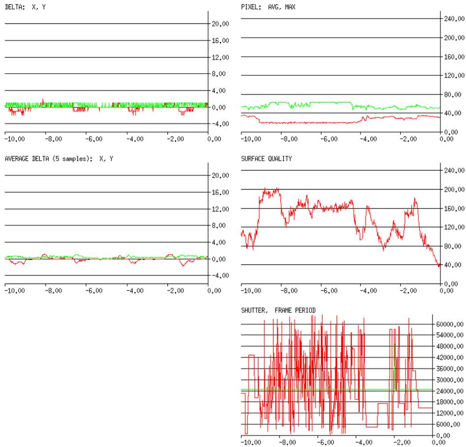
Normal flight with the mouse chip looking down, the measured rates are low, at less than one quanta. Delta X and Y are the motion signals. Quality of the surface (texture) consistently adequate (middle right). Averaging helps increase the signal resolution, at the obvious cost of temporal response (top right).
