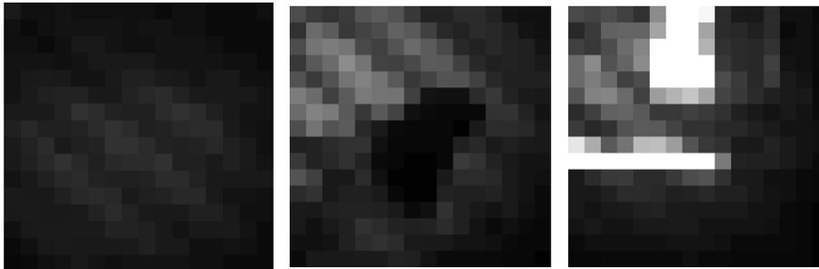
Pixel dumps from the ADNS through “card camera” optics
