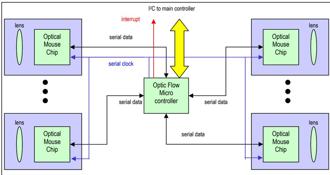
**Figure 5: Local Interconnection Between Optical Flow Microcontroller and Sensor Array**
