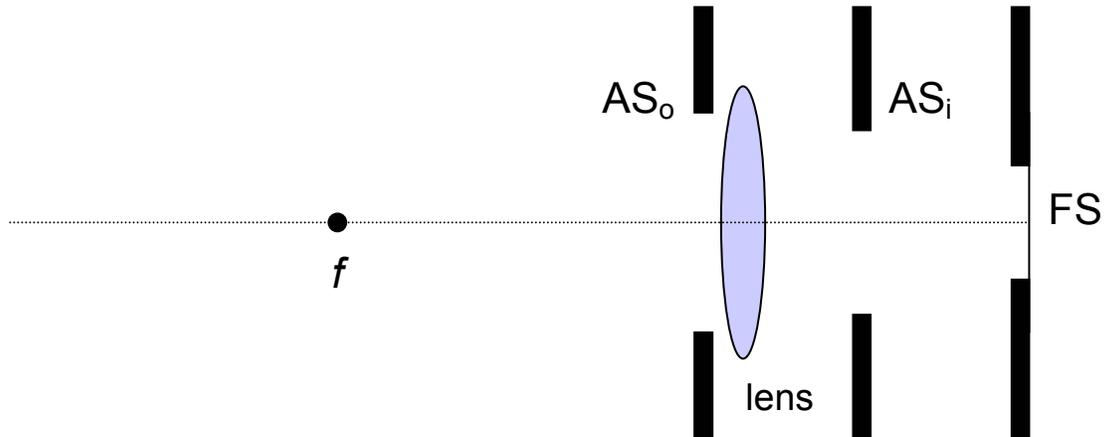
Figure 7: Simple Optical Model Indicating Apertures/Field Stop
