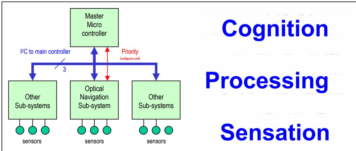
**Figure 4: Overall Control Architecture for Sensor Suite**
