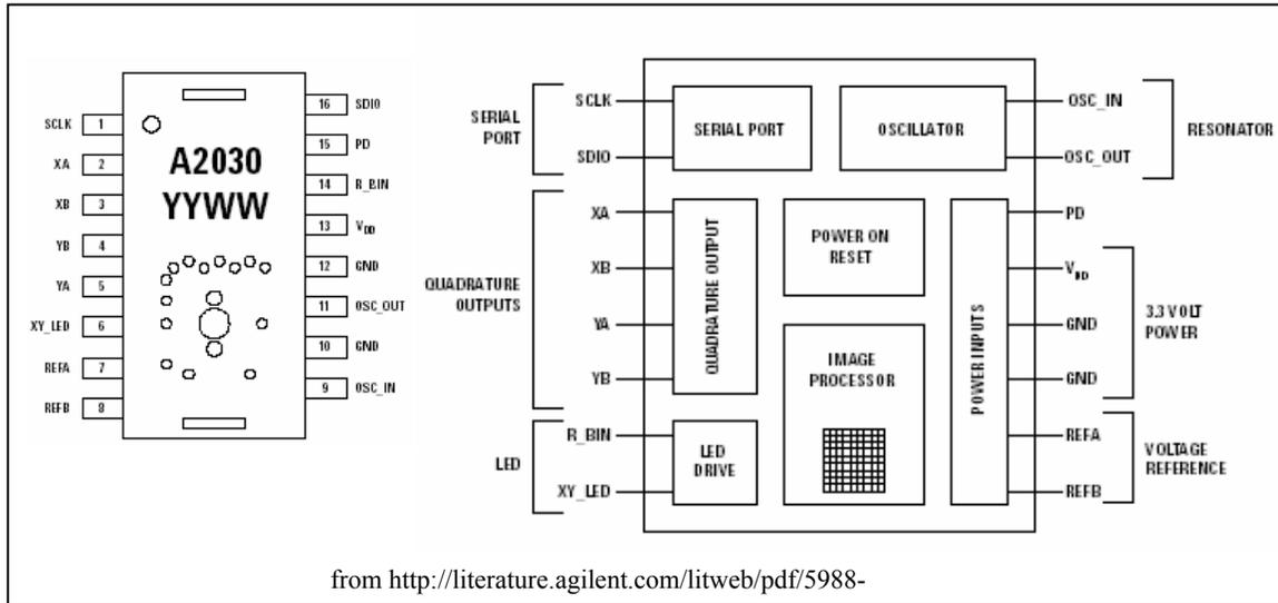
**Figure 3: Optical Mouse Chip Pinout & Block Diagram**
