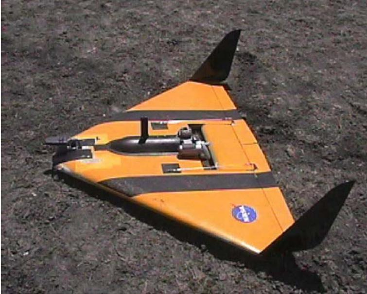
Fig 8: A 5 Kg BEES flyer with Bioinspired sensors embedded in the nose area including the mouse chip adapted optic flow sensor looking downwards on the left in the nose area
