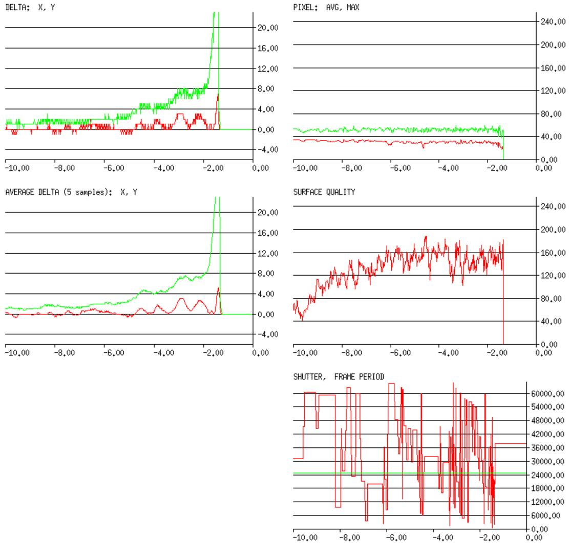
Landing flight. Rates are measurable, and consistent with the landing experience. Rapid increase in rate is apparent at the end of the flight.
