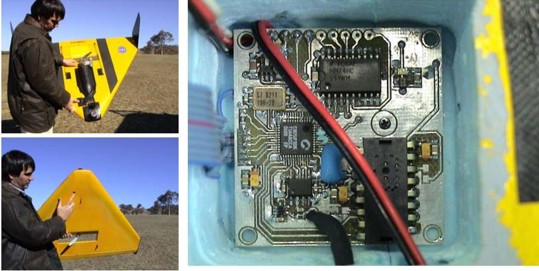
**Top left, port in the wing where the instrument is installed. Bottom left underside of wing showing where the optics looks though the wing. Right the circuit embedded in the wing, major components from top left clockwise crystal (silver), buffer for servo motor drive (inline package), ADNS 2051 (large staggered dip), Cygnal 8051 microcontroller.**
