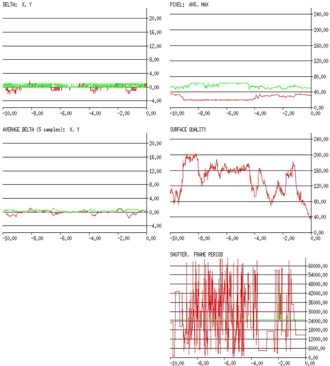
First prototype of the mouse chip. Normal flight with the mouse chip looking down, the measured rates are low, at less than one quanta. Delta X and Y are the motion signals. Quality of the surface (texture) consistently adequate (middle right). Averaging helps increase the signal resolution, at the obvious cost of temporal response (top right).
